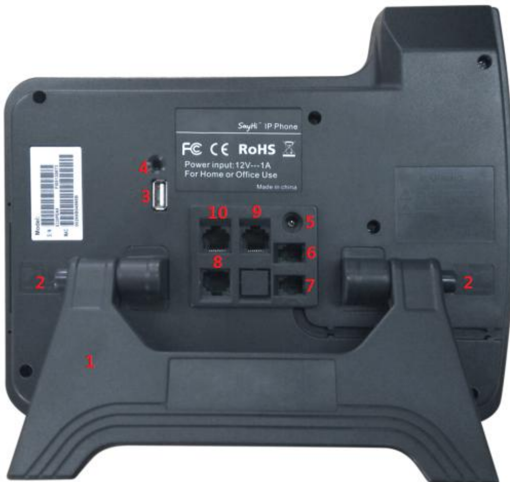
Figure 3.2 Interfaces of SayHi ES330-PEG (NOTE: 330 support expansion, that it has a EXT port)
