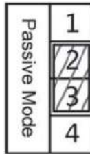
Jumper in passive mode
